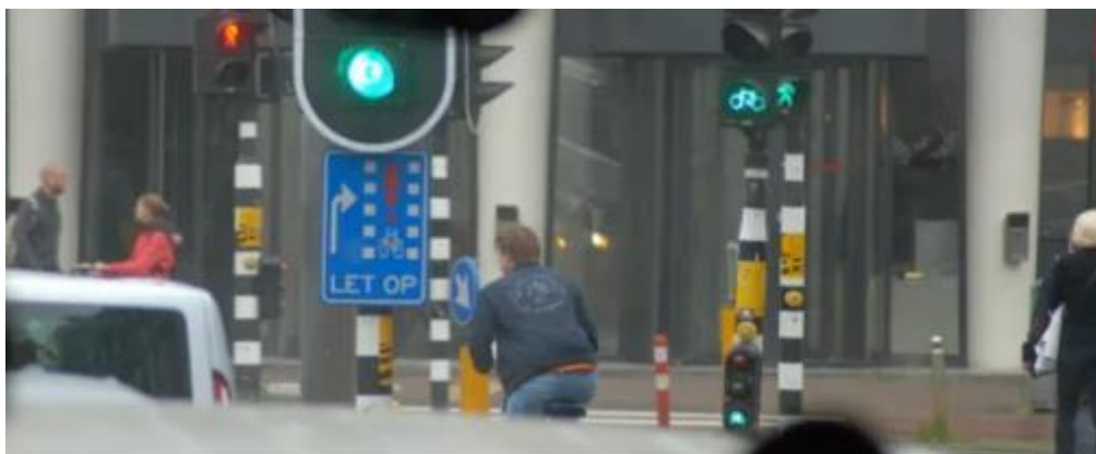
Figure 2.61 Example from the Netherlands of traffic signals + give way signage controlling turning traffic and cyclists (Source: Dutch Design Guide Ontwerprijzer Fietsverkeer)
